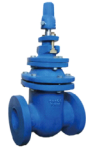
BS CI METAL SEATED GATE VALVE BS664 PN16 AVAILABLE MEDIUM: WATER WORKING TEMPERATURE: ≤50°C FLANGE: BS4504
