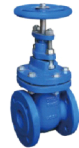
DIN CI NON-RISING STEM GATE VALVE, METAL SEATED, F4 PN16 AVAILABLE MEDIUM: WATER WORKING TEMPERATURE: ≤200 °C FACE TO FACE: DIN3202 F4 FLANGE: DIN2501
