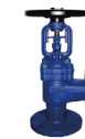
DIN CS ANGLE GLOBE/CHECK VALVE AVAILABLE MEDIUM: WATER, STEAM FACE TO FACE: DIN3202 F32 FLANGE: DIN2533 CLASS: PN10/PN16/PN25/PN40
