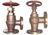
JIS F7302 5K/F7304 16K ANGLE VALVE JIS F7351 5K/F7409 16K ANGLE SDNR VALVE 1.End Type: Flange 2.DN: 15mm-65mm 3.PN: 5K (10K) 16K 4.Design Standard: JISF7400 5.Flange Standard: JISB2220
