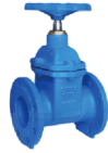
BS CI NON-RISING STEM, RESILIENT SEATED GATE VALVE BS5163 PN16 AVAILABLE MEDIUM: WATER WORKING TEMPERATURE: ≤50°C FLANGE: BS4504
