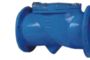
DIN CI CHECK VALVE AVAILABLE MEDIUM: WATER WORKING TEMPERATURE: ≤200 °C FACE TO FACE: DIN3202 F6 FLANGE: DIN2533
