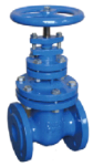
BS CI NON-RISING STEM, METAL SEATED GATE VALVE, BS5163 BS10-TABLE-D AVAILABLE MEDIUM: WATER WORKING TEMPERATURE: ≤120°C FLANGE: BS4504 BS10T/D
