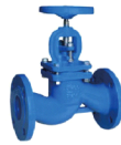
DIN CI GLOBE / CHECK VALVE PN16/PN10 AVAILABLE MEDIUM: WATER WORKING TEMPERATURE: ≤200 °C FACE TO FACE: DIN3202 F1 FLANGE: DIN2533
