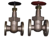
JIS F7367 5K GATE VALVE JIS F7368 10K GATE VALVE 1.End Type: Flange 2.DN: 15mm-65mm 3.PN: 5K 10K 4.Design Standard: JISF7400 5.Flange Standard: JISB2220
