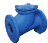
DIN CI BALL CHECK VALVE AVAILABLE MEDIUM: WATER WORKING TEMPERATURE: ≤50 °C FACE TO FACE: DIN3202 F6 FLANGE: DIN2501-PN10
