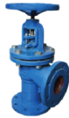
DIN CI ANGLE GLOBE/CHECK VALVE PN16/PN10 AVAILABLE MEDIUM: WATER WORKING TEMPERATURE: ≤200 °C FACE TO FACE: DIN3202 F32 FLANGE: DIN2533
