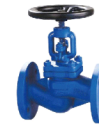
DIN CS GLOBE/CHECK VALVE AVAILABLE MEDIUM: WATER, STEAM FACE TO FACE: DIN3202 F1 FLANGE: DIN2533 CLASS: PN10/PN16/PN25/PN40
