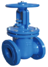
BS CI RISING STEM, METAL SEATED GATE VALVE, BS5163 BS10-TABLE-D AVAILABLE MEDIUM: WATER WORKING TEMPERATURE: ≤120°C FLANGE: BS4504 BS10T/D
