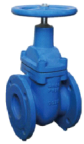
DIN CI NON-RISING STEM GATE VALVE, LIGHT TYPE, PN10 AVAILABLE MEDIUM: WATER WORKING TEMPERATURE: ≤120 °C FACE TO FACE: DIN3202 F4 FLANGE: DIN2501
