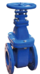
DIN CI METAL SEATED (NON-RISING) GATE VALVE, F4(C) PN16/PN10 AVAILABLE MEDIUM: WATER, STEAM WORKING TEMPERATURE: ≤150 °C FACE TO FACE: DIN3202 F4 FLANGE: DIN2501
