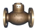
JIS F7356 5K LIFT (ANGLE) CHECK VALVE 1.End Type: Flange 2.DN: 15mm-50mm 3.PN: 5K 4.Design Standard: JISF7400 5.Flange Standard: JISB2220
