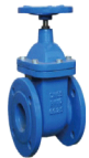
DIN CI NON-RISING STEM GATE VALVE, F4(B) PN16/PN10 AVAILABLE MEDIUM: WATER, STEAM WORKING TEMPERATURE: ≤200 °C FACE TO FACE: DIN3202 F4 FLANGE: DIN2501
