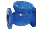
DIN CI SWING CHECK VALVE AVAILABLE MEDIUM: WATER WORKING TEMPERATURE: ≤200 °C FACE TO FACE: DIN3202 F6 FLANGE: DIN2533
