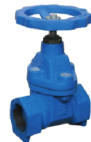
DIN CI RESILIENT GATE VALVE, THREAD ENDS, PN16/PN10 AVAILABLE MEDIUM: WATER WORKING TEMPERATURE: ≤50 °C SCREWED: BSP
