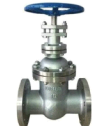
DIN CS GATE VALVE AVAILABLE MEDIUM: WATER, STEAM FACE TO FACE: DIN3202 FLANGE: DIN3352 CLASS: PN10/PN16/PN25/PN40
