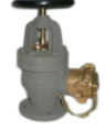
JIS F7333A(B) 5K/10K CAST IRON HOSE (ANGLE) VALVE 1.End Type: Flange 2.DN: 50mm/65mm 3.PN: 5K 10K 4.Design Standard: JISF7400 5.Flange Standard: JISB2220
