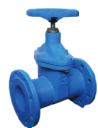
DIN CI NON-RISING STEM GATE VALVE, RESILIENT SEATED, F5 PN16 AVAILABLE MEDIUM: WATER WORKING TEMPERATURE: ≤50 °C FACE TO FACE: DIN3202 F5 FLANGE: DIN2501
