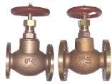
JIS F7301 5K/F7303 16K GLOBE VALVE JIS F7351 5K/F7409 16K SDNR VALVE 1.End Type: Flange 2.DN: 15mm-65mm 3.PN: 5K (10K) 16K 4.Design Standard: JISF7400 5.Flange Standard: JISB2220
