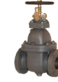
JIS F7363 5K/F7364 10K CAST IRON GATE VALVE 1.End Type: Flange 2.DN: 50mm-600mm 3.PN: 5K 10K 4.Design Standard: JISF7400 5.Flange Standard: JISB2220
